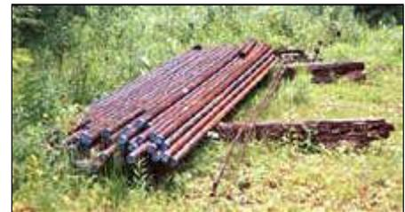
*Pulled 2" pipe at a recently plugged and abandoned oil well. This is the type of equipment sampled for NORM*
